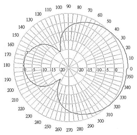
STR-3 antenna RHCP response / ANTENNA RADIATION PATTERN TEST
